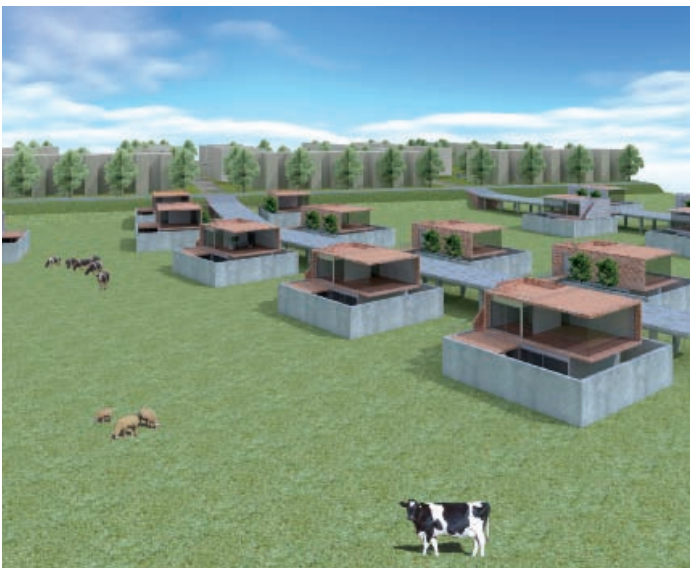
Watergaten (Waterholes) project, 's-Hertogenbosch, Runday Winkelaar Architects The Waterhole houses do not employ conventional foundations but instead respond to fluctuating water levels. www.rundaywinkelaar.nl
